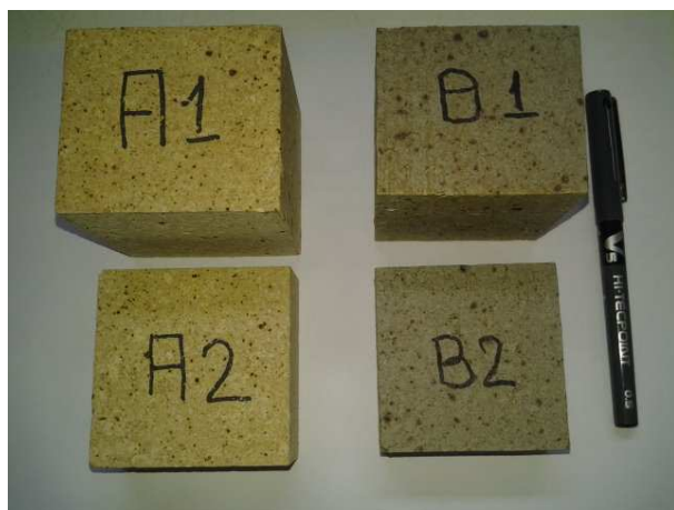
Figure 6 : Image of fired bricks : A- 1400 and B- 1500°C
